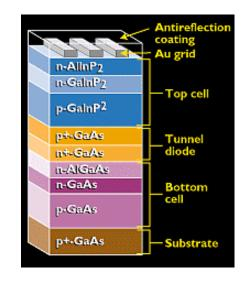
Much of today's research in multi junction cells focuses on gallium arsenide as one (or all) of the component cells. Such cells have reached efficiencies of around 35% under concentrated sunlight. Other materials studied for multi junction devices have been amorphous silicon and copper indium diselenide.
